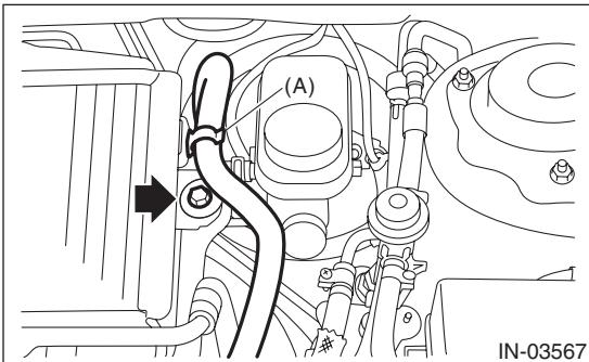
6) Tighten the bolt securing the intercooler stay LH to the intake manifold.
