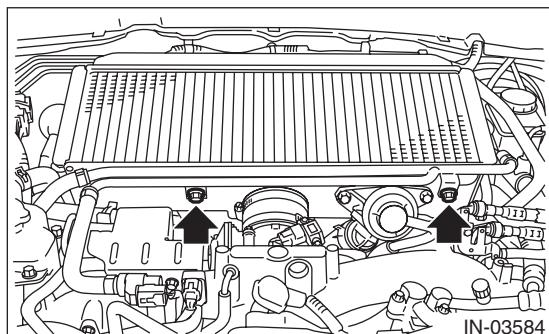
11) Install the chamber assembly. <Ref. to IN(STI)-22, INSTALLATION, Chamber Assembly.>
