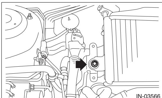
4) Temporarily tighten the bolt securing the intercooler stay LH to the intake manifold.
