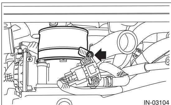
3) Set the intercooler to the vehicle, and install the bolts securing the intercooler to the intercooler stay RH No. 1.
