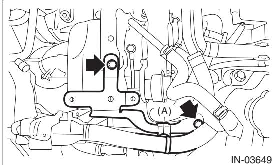
2) Attach the air duct hose to the throttle body.
