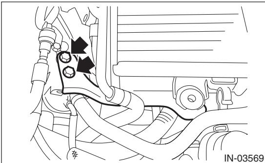
5) Install the bolts which secure the intercooler to the intercooler stay LH, and install the brake booster vacuum hose to the clip (A).
