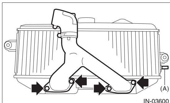
2) Remove the intake duct from intercooler duct.
