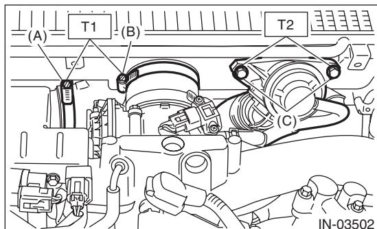
10) Install the PCV pipe to the intercooler.
