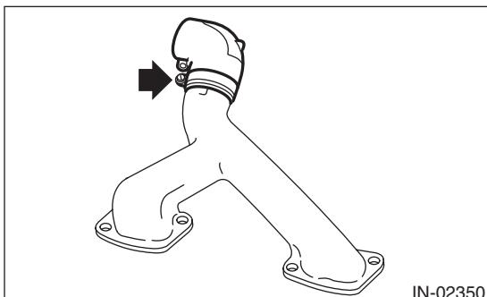
2) Install the clip (A) and intercooler duct to the intercooler.
